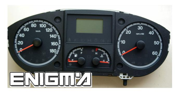
Use cable C4, open all dash, please make it carefully, locate eeprom memory 95040 and clip it checking PIN 1 as shown of photo below:
