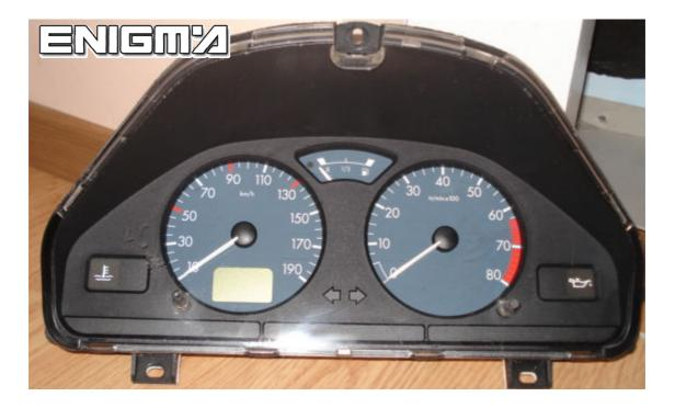
USE SPECIFIC CABLE C21, TAKE OFF DASH FROM CAR, CONNECT PLUG TO DASH LIKE WE CAN SEE ON NEXT PHOTO AND RUN PROGRAM:
