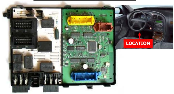
USE CABLE C13 ALWAYS CONNECTED TO A1 ADAPTER. TAKE OFF BOTH SIDES FROM BSI, THEN CONNECT OR SOLDER CABLE LEADS ACCORDING TO NUMBER AS SHOWN OF BELOW PHOTO(WE MUST DESOLDER TRANSISTOR FROM LEAD 9 AND UP PIN 10):
