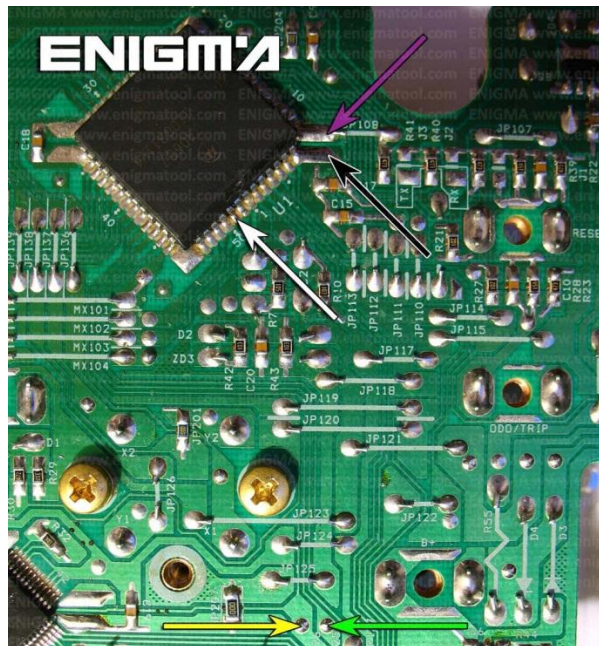
PHOTO 1: Solder C11 cables according to the colors like shown on the photos above.
