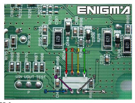
**PHOTO 1:** Solder cable C7 to points according to the picture above.
