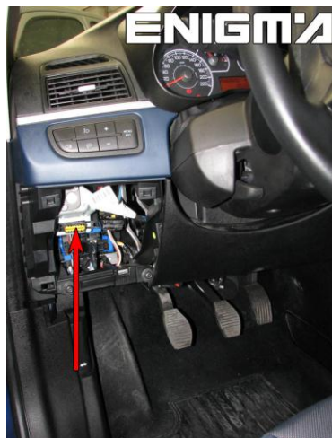
PHOTO 1: Connect cable C1+A9 adapter as shown on the picture above.
