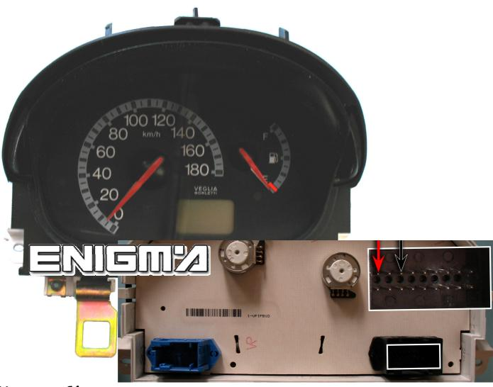
USE CABLE C4, OPEN ALL DASH, PLEASE MAKE IT CAREFULLY, THEN LOCATE EPROM MEMORY, AND CLIP IT CHECKING PIN 1 AS SHOWN OF PHOTO BELOW:
