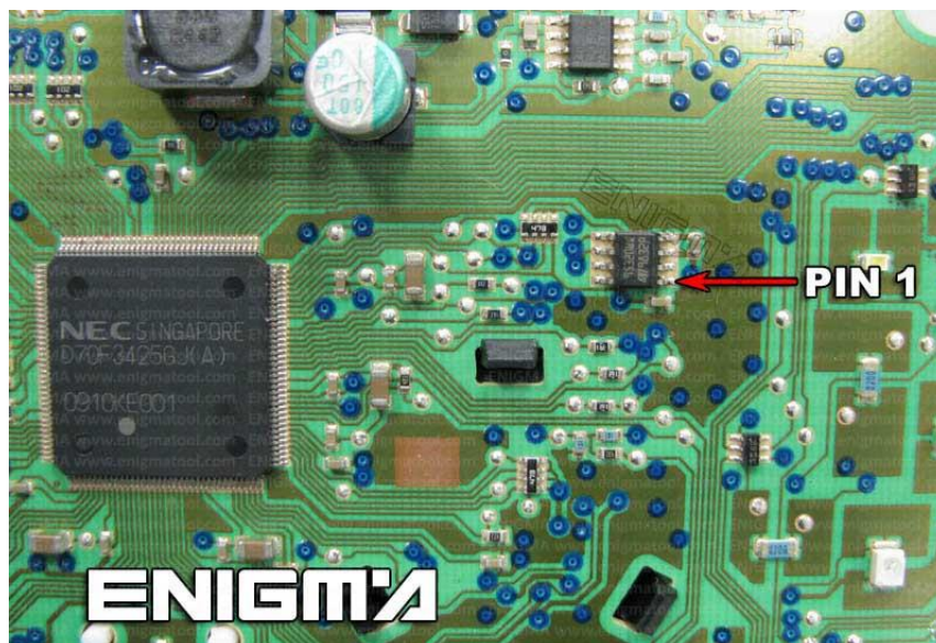
PHOTO 1: Connect cable C4 to the EEPROM memory according to the picture above.
