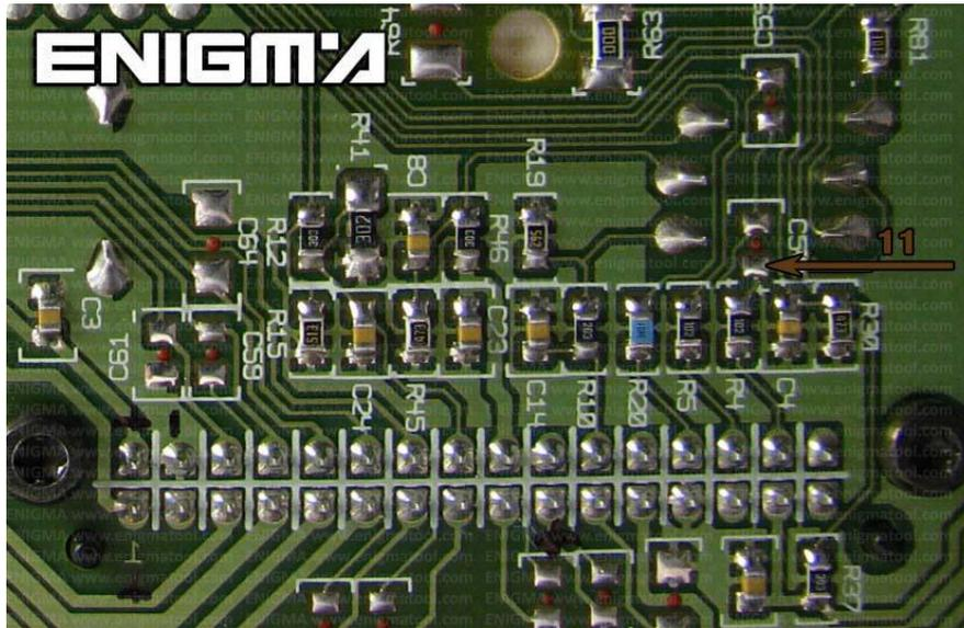
**PHOTO 3:** Solder C13 cable like shown on photo above.
