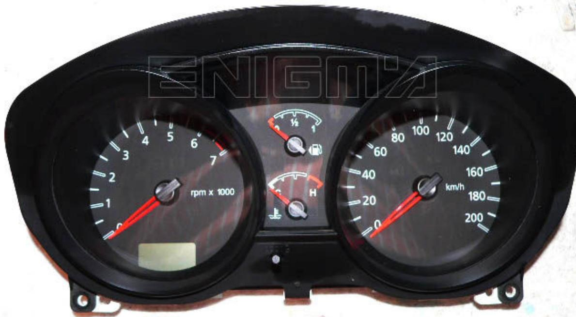
USE CABLE C4, OPEN ALL DASH, PLEASE MAKE IT CAREFULLY, THEN LOCATE EPROM MEMORY, AND CLIP IT CHECKING **PIN 1** AS SHOWN OF PHOTO BELOW:
