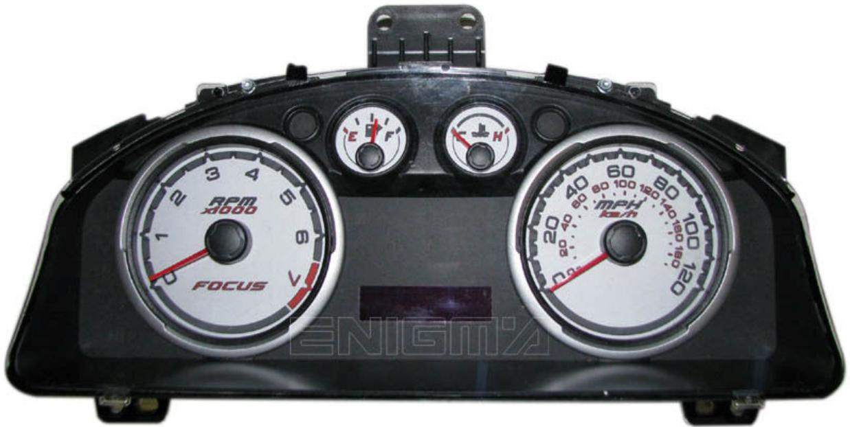
USE CABLE C12, REMOVE BACK PLASTIC COVER, YOU HAVE TO LOOK FOR POINTS ON THE MAIN BOARD AND SOLDER CABLE LEADS ACCORDING TO COLOURS AS SHOWN ON BELOW PHOTO:
