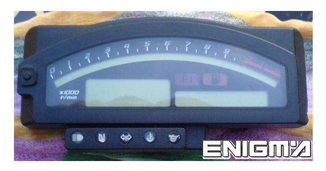
USE CABLE C4, OPEN BACK SIDE OF DASH, CAREFULLY, THEN LOCATE EPROM 93C56 MEMORY, AND CLIP IT CHECKING PIN 1 AS SHOWN OF BELOW PHOTO:
