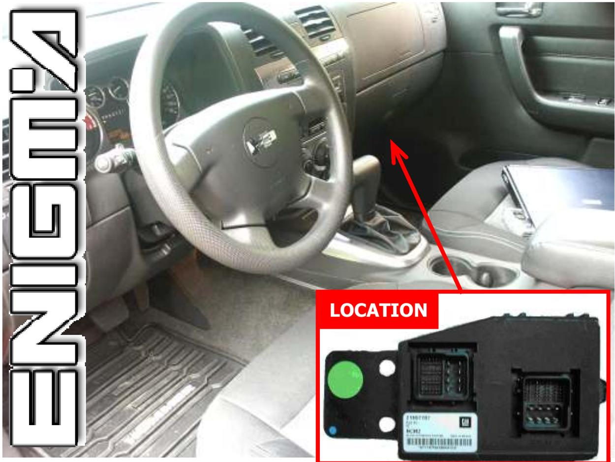
REMOVE BCM FROM CAR, OPEN COMPLETELY, USING CABLE C4 LOCATE EEPROM 95040 AND CLIP IT CHECKING PIN 1 AS SHOWN OF BELOW PHOTO:
