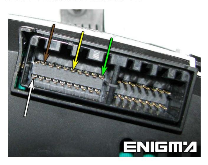
WE ALSO CAN USE CABLE C4, OPEN CAREFULLY ALL DASH, THEN LOCATE EPROM 93S56 MEMORY, AND CLIP IT CHECKING PIN 1 AS SHOWN ON PHOTO BELLOW:
