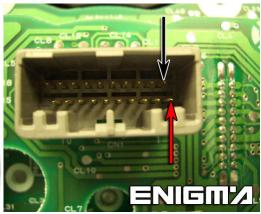
USE CABLE C4, REMOVE BACK PLASTIC COVER FROM DASH, AND THEN LOCATE EPROM AND CLIP
