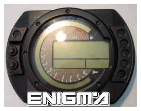
USE CABLE C4, OPEN BACK PLASTIC COVER FROM DASH, CAREFULLY REMOVE UPPER BOARD, THEN LOCATE EPROM MEMORY, AND CLIP IT CHECKING PIN 1 AS SHOWN INTO BELOW PHOTOS:
