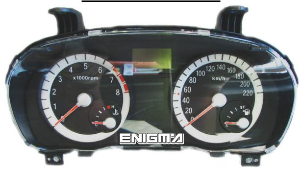
Use cable C4, open dash completely, please make it carefully, then locate eeprom 93S56 memory and clip it checking Pin 1 as shown of photo below:
