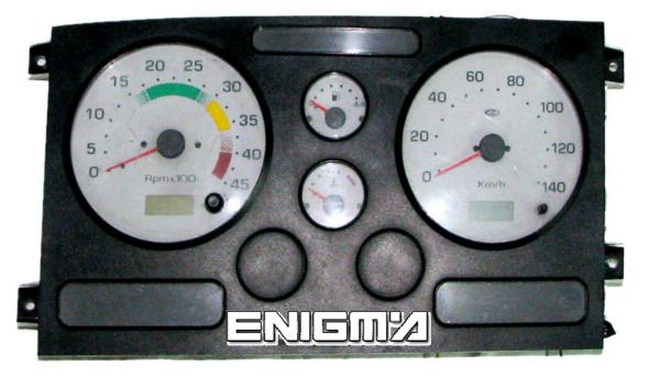
USE CABLE C12, REMOVE DASH FROM CAR, OPEN DASH, PLEASE MAKE IT CAREFULLY. TAKE OFF ONLY SPEEDOMETER, WHEN WE HAVE MAIN BOARD ON OUR HANDS SOLDER CABLE LEADS ACCORDING TO COLOURS AS SHOWN ON THE PHOTOS BELOW:
