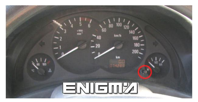
AFTER REPROGRAMATION DISCONNET THREE FUSES (YOU CAN SEE WHICH ONES ON NEXT PICTURE) FOR AROUND 15 SECONDS AND CONNECT IT BACK.
