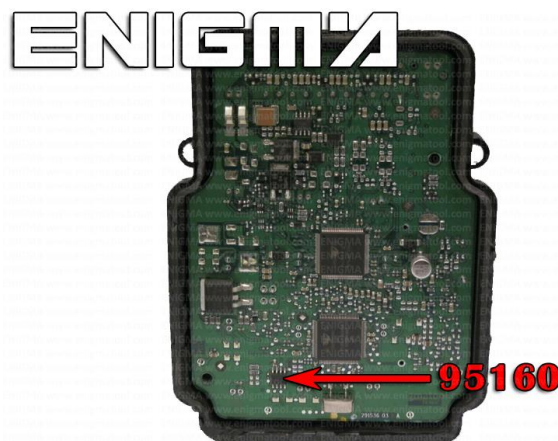
PHOTO 1: Find 95160 EEPROM memory like shown on the photo above.
