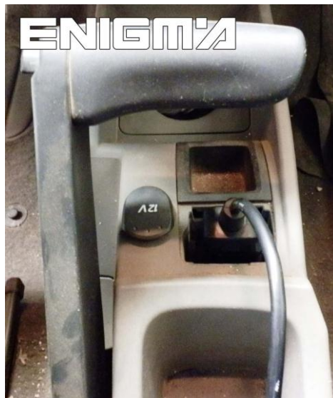
PHOTO 1: Connect cable C1 as shown on the picture above.
