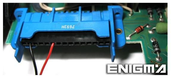
THEN CONNECT OR SOLDER CABLE LEADS ACCORDING TO COLOURS AS SHOWN ON THE PHOTO BELOW, REMEMBER TO LIFT UP PIN FROM WHITE LEAD:
