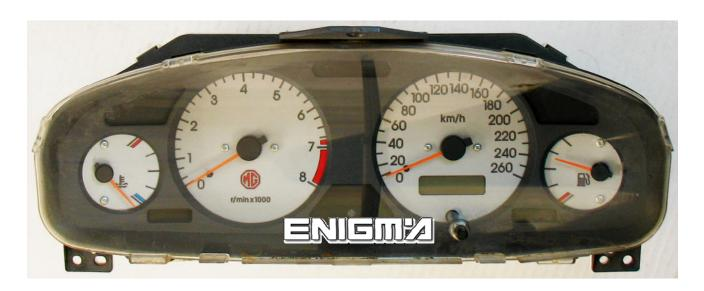
Use cable C4, remove dash from car, open dash, and please make it carefully. Take off now only spedometer, it is the screen one, now locate eprom 93C46 memory, and clip it checking pin 1 as shown of photo below:
