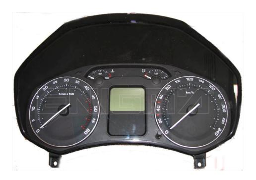
Use cable C4, remove dash from car and open it completely. Separate both boards from dash. Check if MICRO in dash is MICRONAS 3272, then locate eprom 24C32 and clip it checking PIN 1 as shown of below photo:
