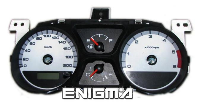
Use cable C4, open all dash, but we must take MUCH carefully, we must take off nails, then locate eprom L56 memory, and clip it checking pin 1 as shown of below photo:
