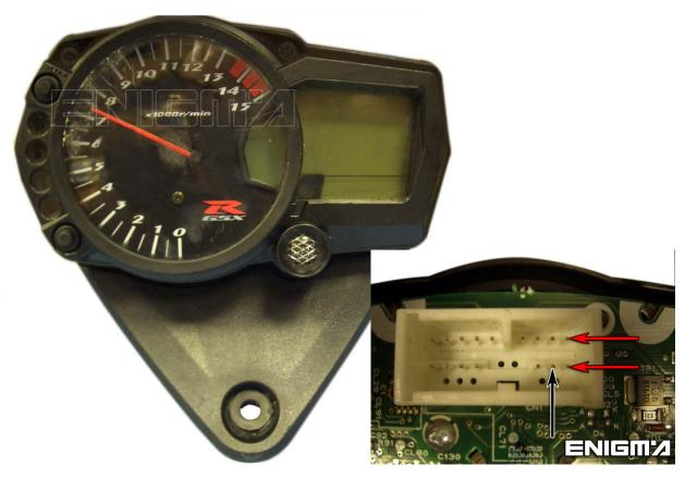
USE CABLE C4, REMOVE BACK COVER, CAREFULLY, THEN LOCATE RL56 EEPROM, AND CLIP IT CHECKING PIN 1 AS SHOWN OF PHOTO BELOW:
