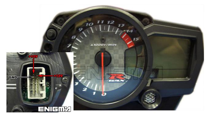
USE CABLE C4, REMOVE BACK COVER, CAREFULLY, THEN LOCATE 93C56 EEPROM, AND CLIP IT CHECKING PIN 1 AS SHOWN ON PHOTO BELOW:
