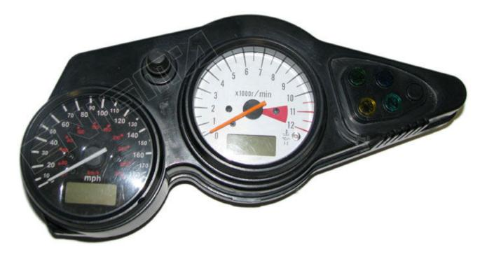
USE CABLE C7, OPEN BACK DASH COVER, THEN LOCATE POINTS ON THE MAIN BOARD, AND THEN SOLDER CABLE LEADS CONCORDANCE WITH ITS NUMBER-COLOUR:
