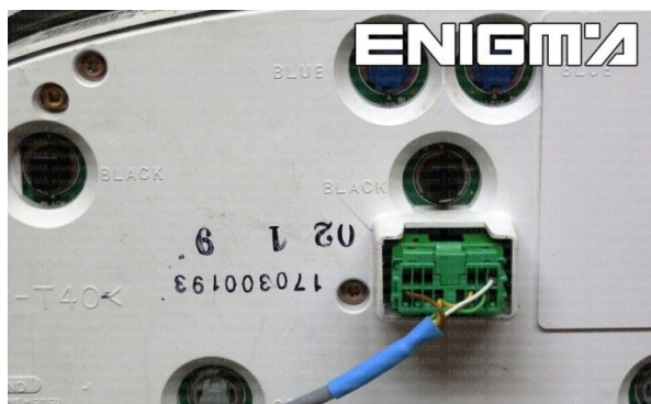
PHOTO 1: Connect cable C41 according to the colors like shown on the photo above.
