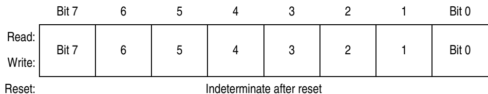
Figure 22-15. TIM Channel 1 Register Low (TCH1L)
