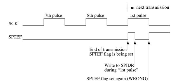
Then the SPTEF flag is set at the falling SCK edge of the "1st pulse" and data is transferred from the SPI Data Register to the transmit shift register. The result is that the transmission is corrupted and data is lost.
