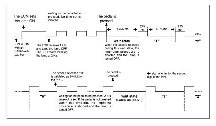
5. After correct code entry the lamp blinks (0.5 Hz) to indicate to the user to switch the ignition off and on again, so that the ICU and ECM can communicate and "unlock" the engine.
