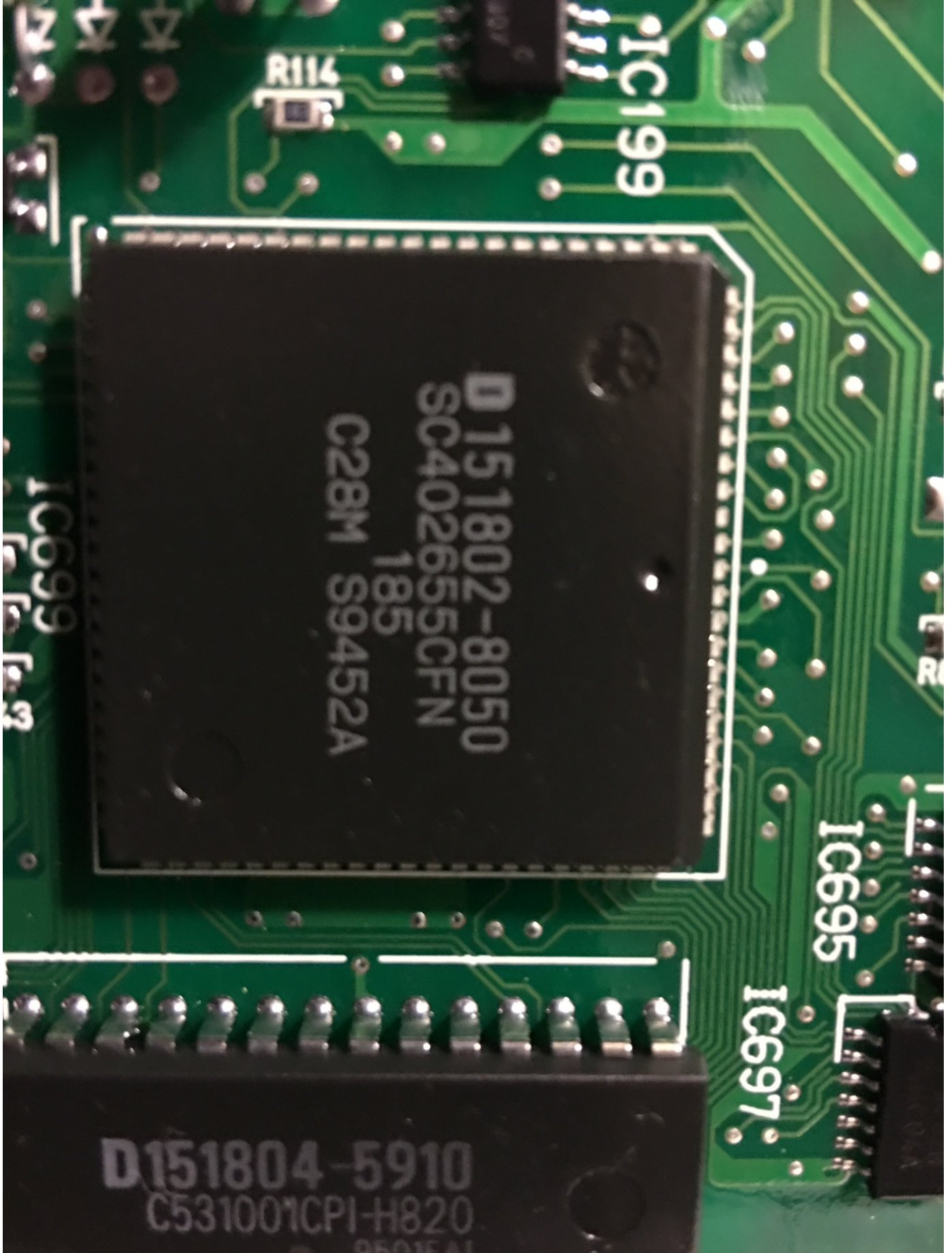
Figure 1. IC699 points to the CPU of the board
