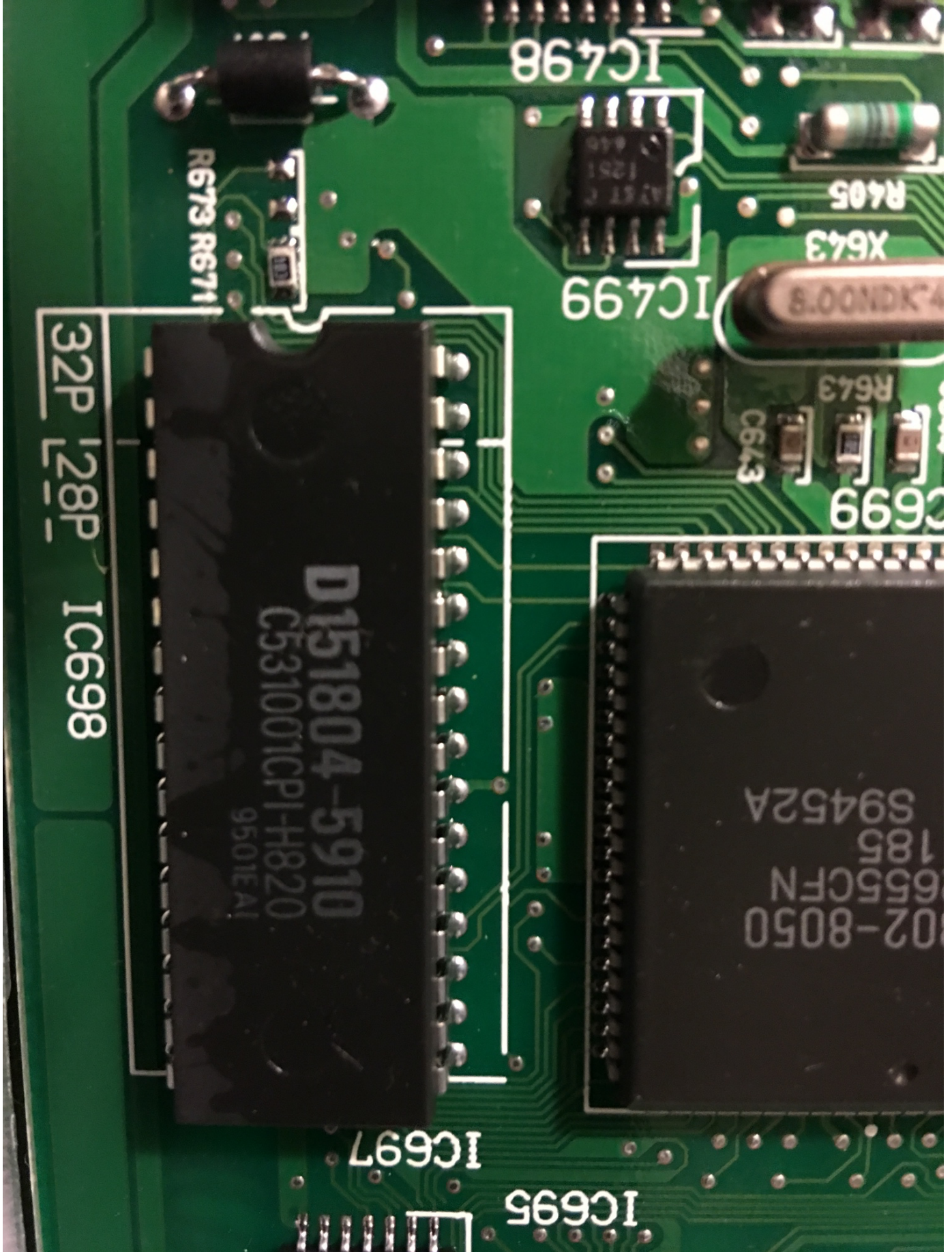
Figure 2. IC698 points to the EPROM on the board
