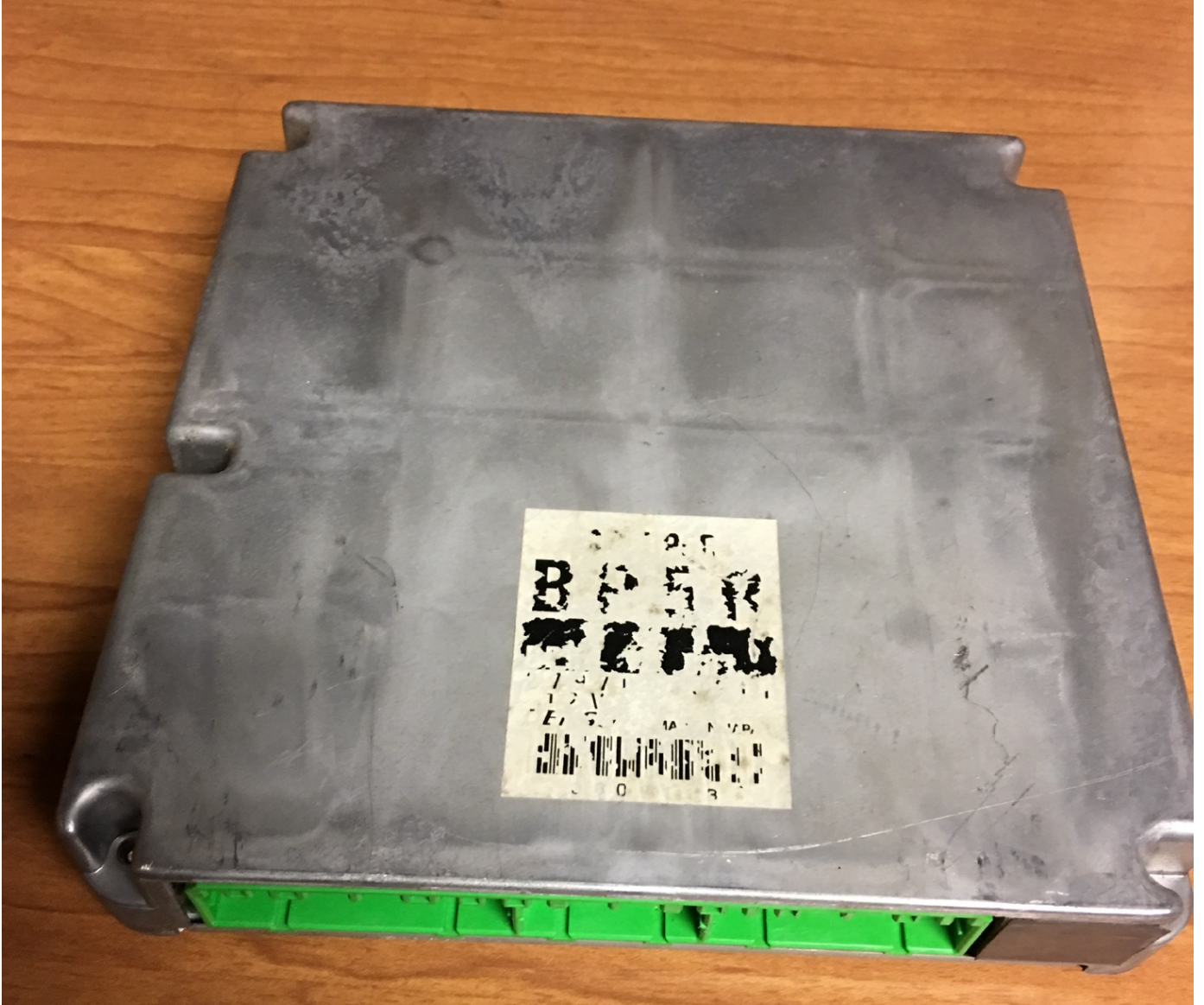
Figure 1. The ECU is enclosed in a secure aluminum box
