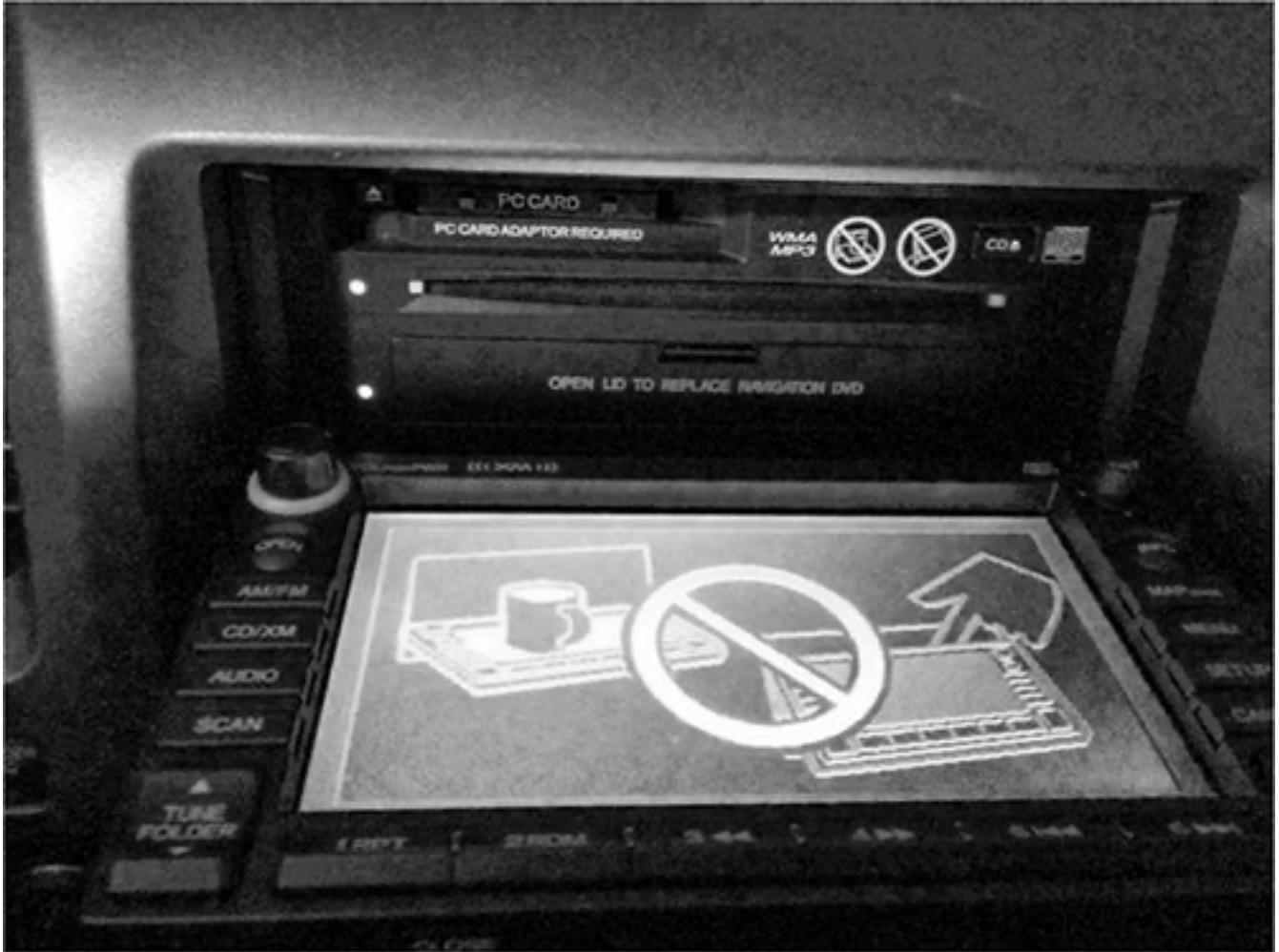
Figure 9-1: NavTeq infotainment unit in an open state
