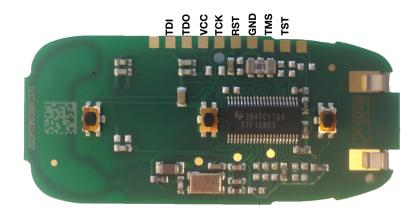
**Figure 3:** The Tesla Model S key fob PCB with the TMS37F128 chip in the middle. The square shaped pads at the top can be used to connect an MSP430 compatible JTAG debugger.
