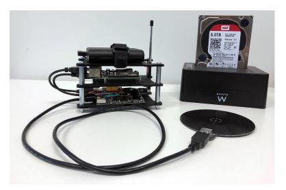
**Figure 6:** The entire attack platform. Consisting of a Yard Stick one, Proxmark III, Raspberry Pi 3 Model B+, a battery pack and a 6 TB hard drive.
