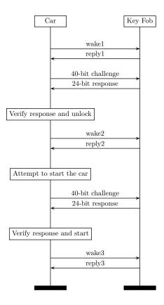
**Figure 4:** The PKES protocol during nominal operation assuming the key fob is in range of the car.
