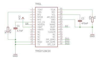
**Figure 8:** The correct pinout for the TMS37126 ICs we tested and an example schematic of how to connect it to an Arduino Pro Mini.
