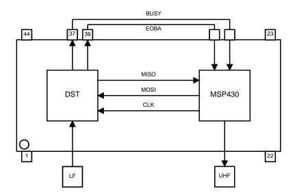
**Figure 7:** A schematic overview of the TMS37F128 package with the DST co-processor and MSP430 microcontroller. During nominal operation a challenge is receiver over LF and communicated to the MSP430 using the EOBA pin. Afterwards, the microcontroller sends it to the transponder over SPI after which it transmits the returned response over UHF.
