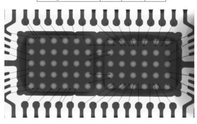
**Figure 2:** X-ray image of the Texas Instruments TMS37F128. From this image one can identify two dies interconnected by five bond wires. Better viewed on-screen.
