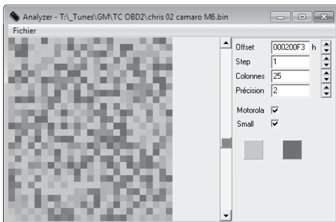
Figure 6-8: This random code doesn't have the neat, orderly patterns that are present in most tables.
